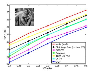
Fig. 2: PSNR comparison of various algorithms for compressive sensing with wavelet-based image representation.
