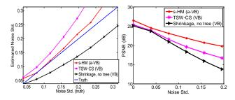
Fig. 4: Left: inferred noise standard deviation plotted versus truth. Right: reconstructed PSNR of "Barbara" with different algorithms, at CS ratio = 0.4 under various noise levels.
