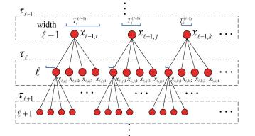
Fig. 1: Depiction of the layers of the trees, with  $n_c = 4$  children considered. Note that each parent coefficient at layer  $\ell - 1$  has a relative width  $T_i^{(\ell-1)}$ , and all widths at a given layer sum to one. The width of the parent is partitioned into windows of width  $T_i^{(\ell-1)}/n_c$  for the children.
